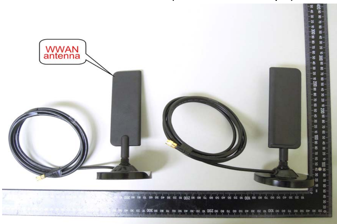
WWAN External Antenna-4 (Part No.: TG.30.8111 Apex)
