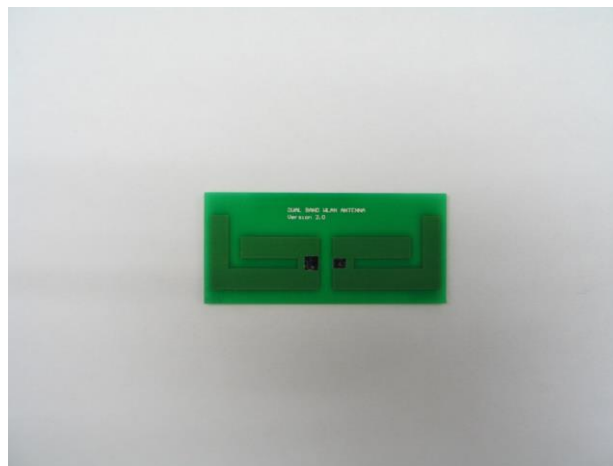
Figure 1 WIFI Internal Dual Band Antenna
