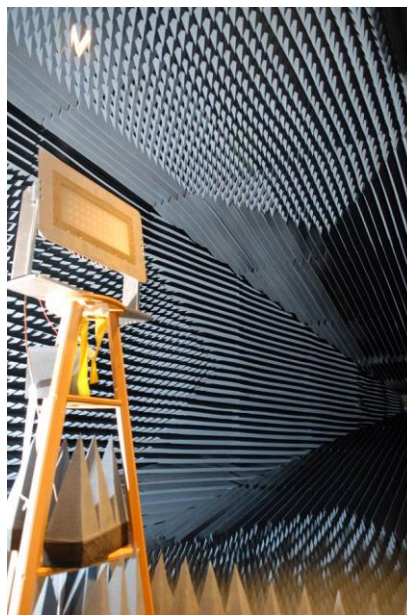
Figure 12 Interior View of the Full Anechoic Chamber
