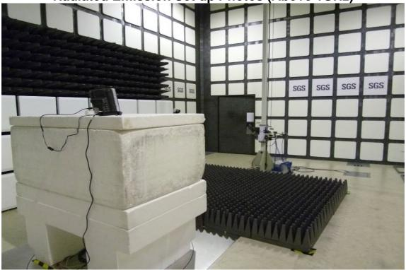
Radiated Emission Set up Photos (Front View)
