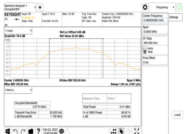
OBW_BLE 2M_HighCH39-2480MHz
