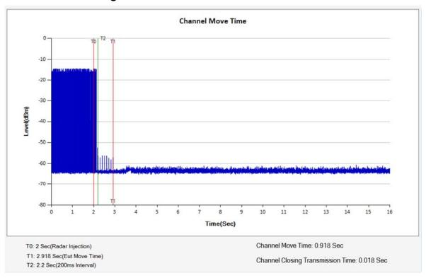
**Verdict:** Note: narrowing the sweep time as the good engineering process for the verification of transmission closing in 200ms
