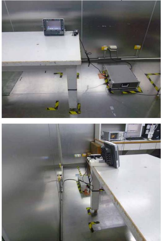
AC Power-line Conducted Emission Set up Photo
