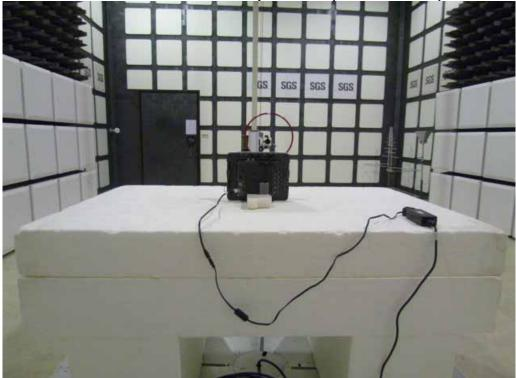
Radiated Emission Setup Photos (30MHz~1GHz)
