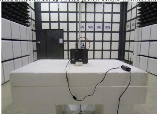
Radiated Emission Set up Photos (Below 1GHz\_Internal Antenna)
