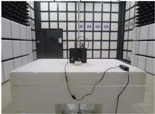
Radiated Emission Set up Photos (Below 1GHz\_External Antenna)
