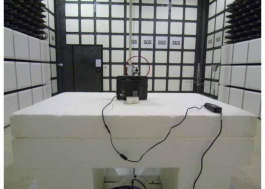
Radiated Emission Set up Photos (Below 1GHz\_Internal Antenna)
