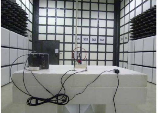
Radiated Emission Set up Photos (Below 1GHz\_External Antenna)
