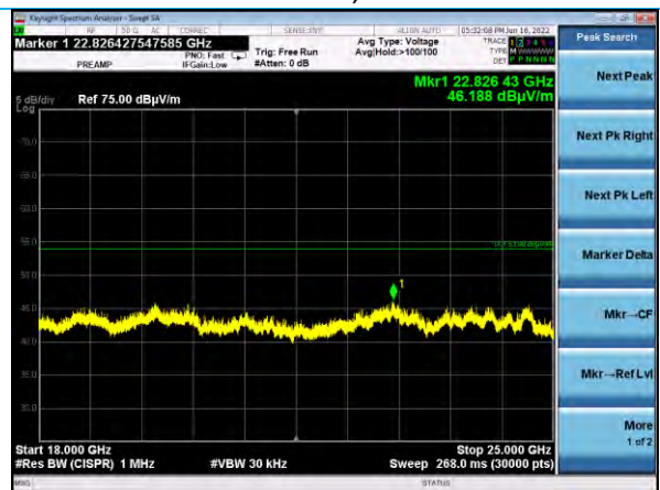
18-25 GHz, Vertical Antenna Flat EUT, Channel 38
