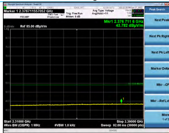
3-DH5 2.31-2.39 GHz, Vertical Antenna Horizontal EUT, Hopping Average
