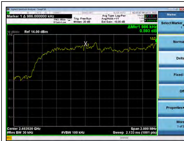
Channel Frequency Delay Separation, EDR3
