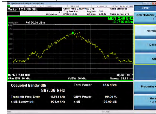
99% Occupied Bandwidth, Channel 78
