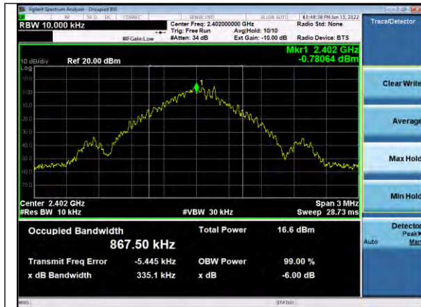
99% Occupied Bandwidth, Channel 0
