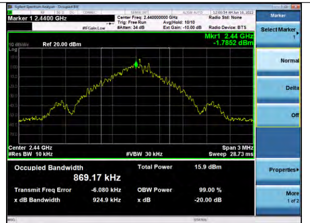
99% Occupied Bandwidth, Channel 38
