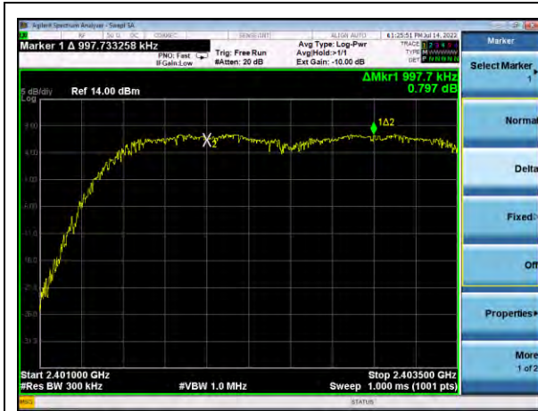
Channel Frequency Separation, EDR2
