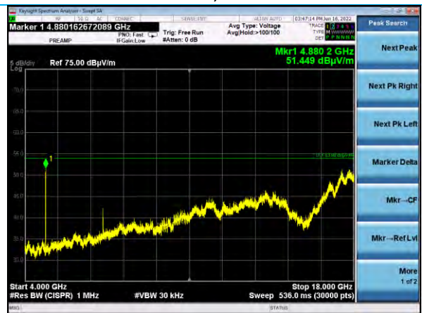
4-18 GHz, Vertical Antenna Horizontal EUT, Channel 38
