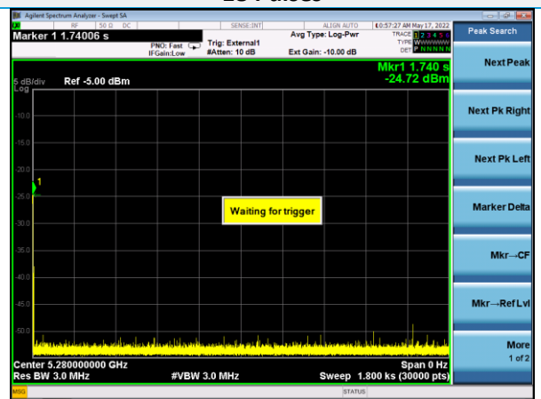
30 Minute Non-Occupancy Period – “Waiting for trigger” message appeared after the Non-Occupancy Period
