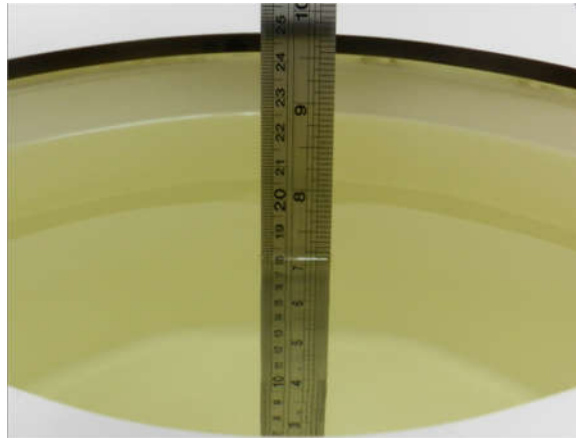
Fig 11.1 Photo of Liquid Height for Body SAR
