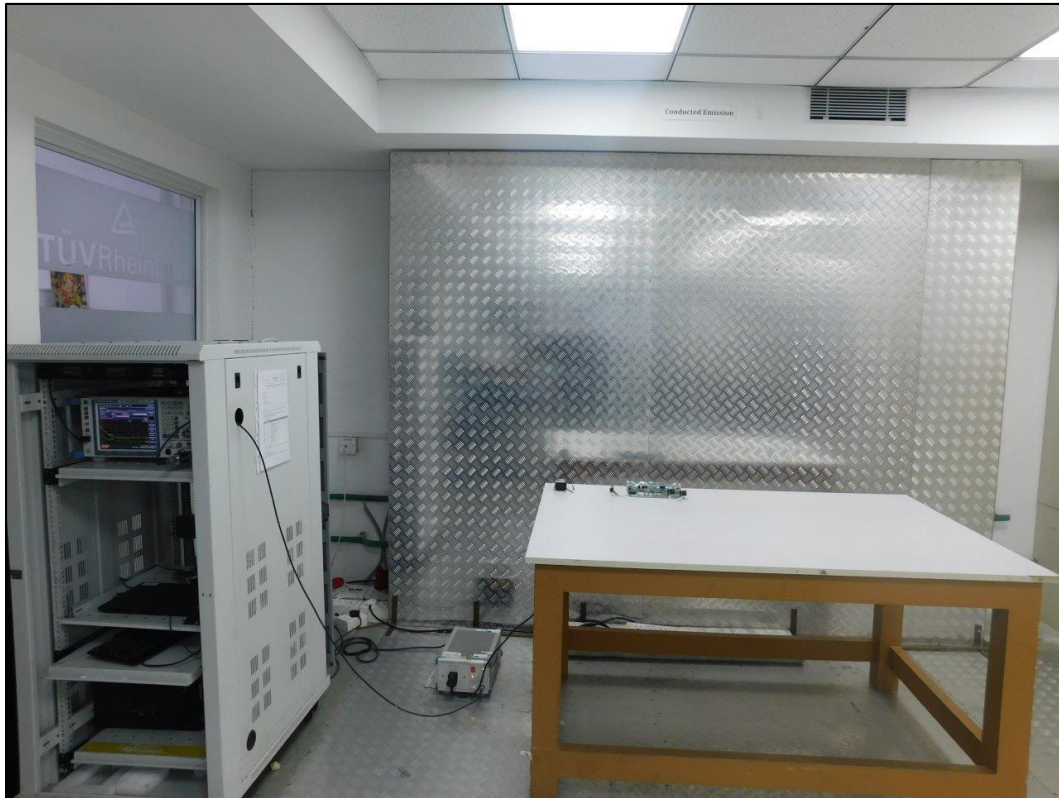
Conducted AC Powerline Test Setup
