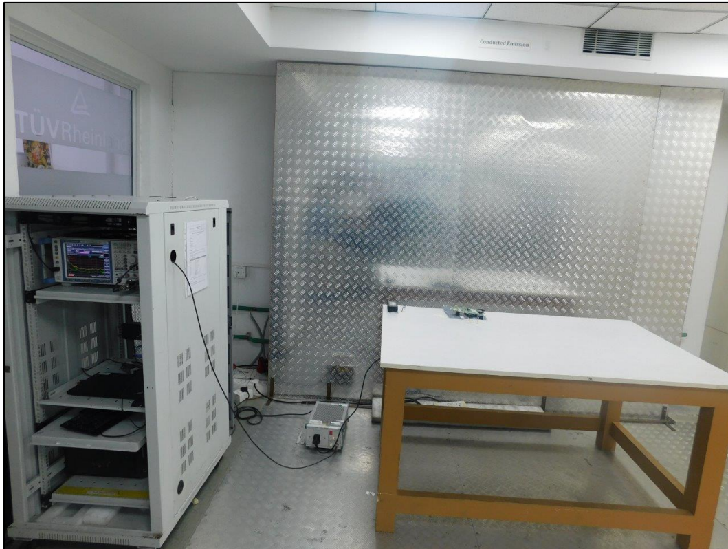
Conducted AC Powerline Test Setup
