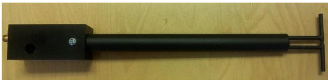
Figure 1 – MVG COMOSAR Validation Dipole
