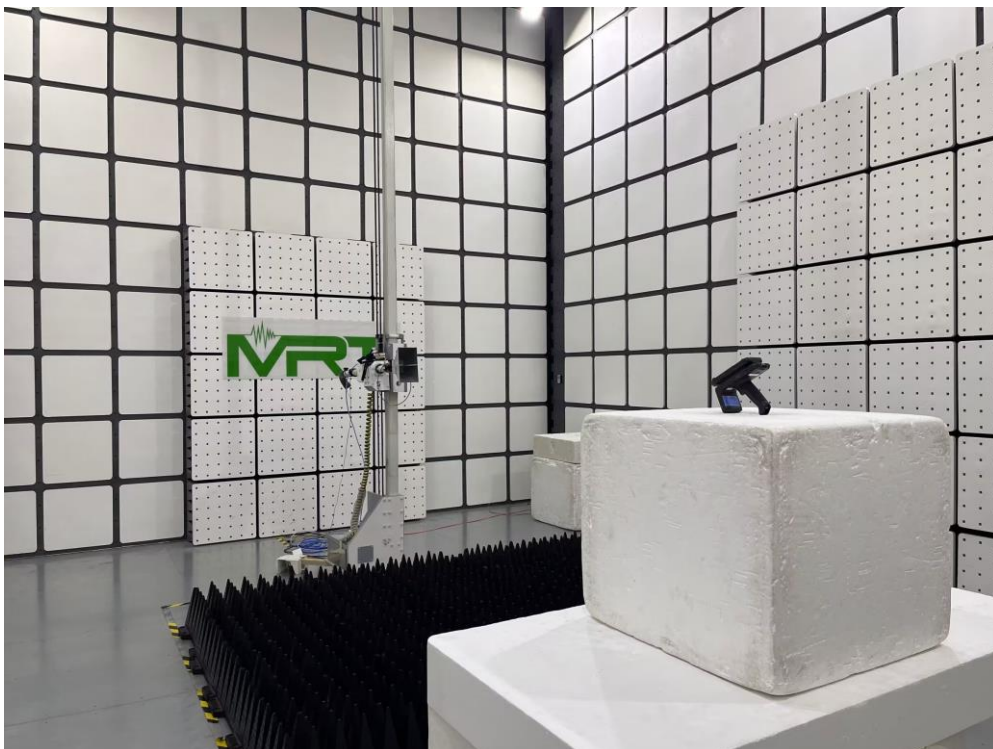
Description: Radiated Spurious Emission Test Setup for Above 1GHz - RFID
