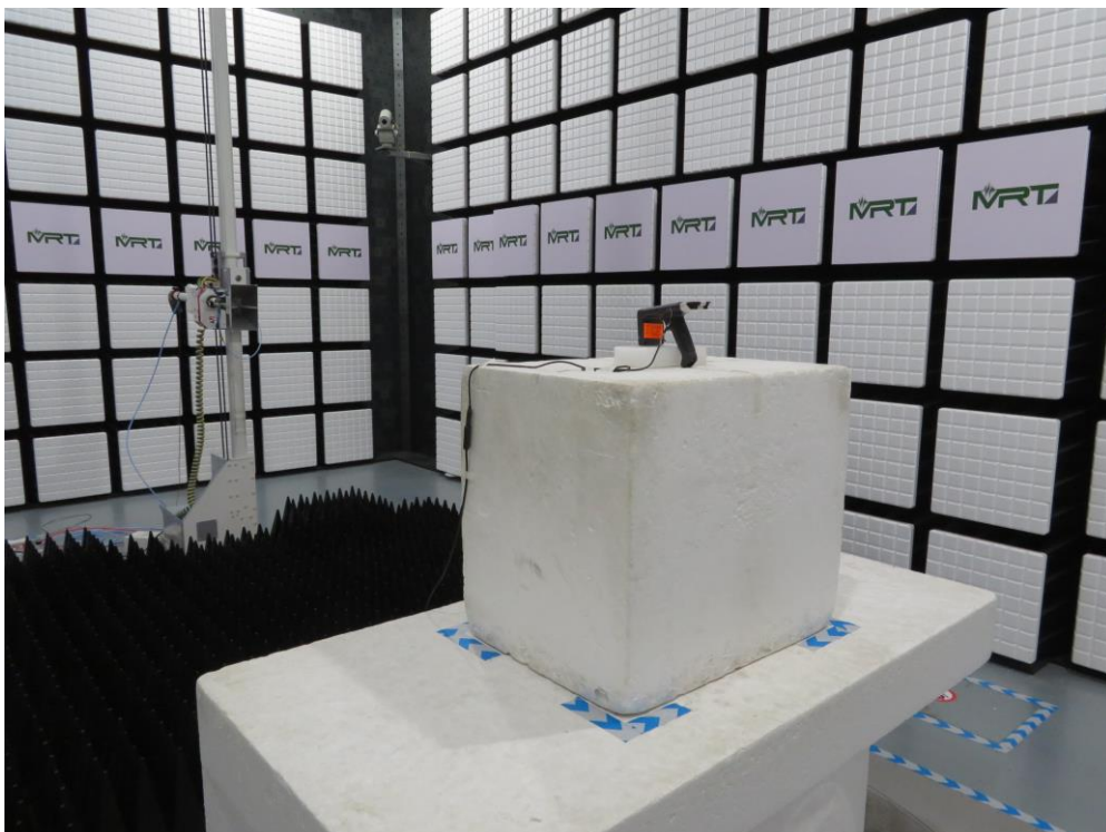
Description: Radiated Spurious Emission Test Setup for Above 1GHz - BT
