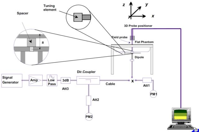
System Performance Check Setup Diagram
