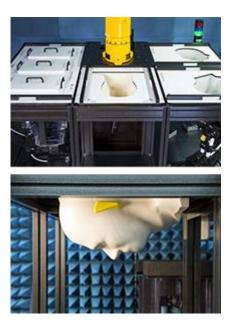
The SAM Head Stand Phantom V10 allows assessment of the exposure of the top-head or around-the-head wireless accessories, e.g., head-belts, etc. It is manufactured from high precision injection molded polypropylene. The Mounting Device for Transmitters including extensions kit can be used to position the device.
