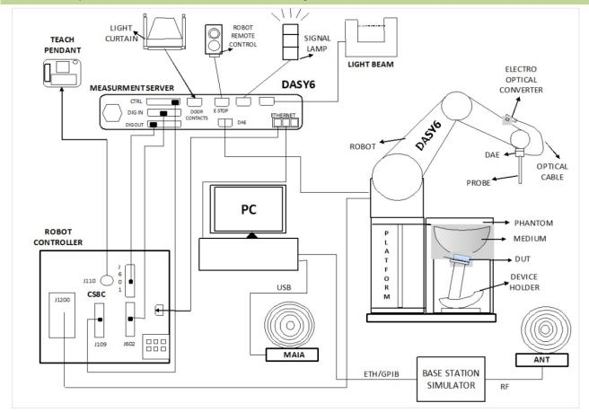
The DASY6 system in cDASY6/DASY5 V5.2 SAR Configuration is shown below:
