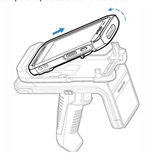
3. To remove the bracket, hold the handle with one hand and lift the bracket up from the RFID Reader with the other hand
