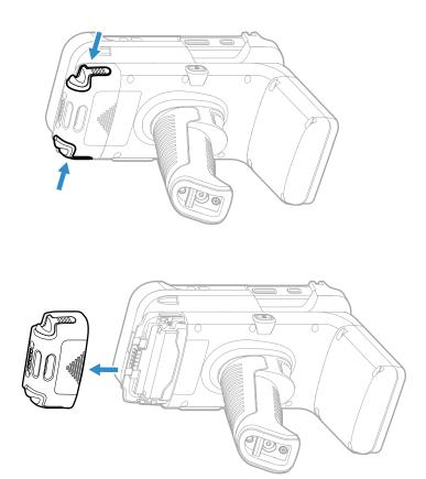
2. Insert the battery into the battery compartment.
