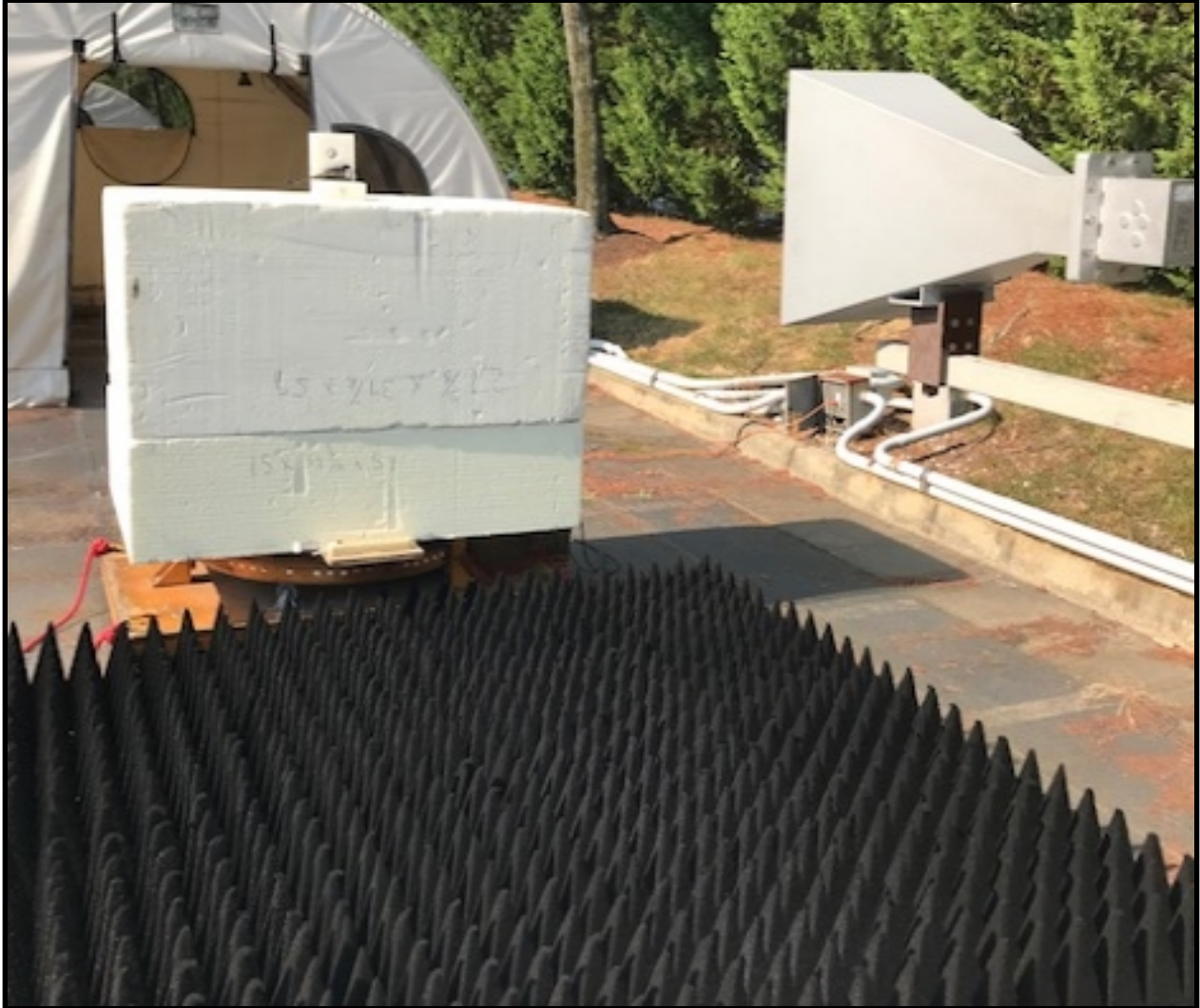
Photograph 1: Radiated Emissions Testing – Front View (Above 1 GHz)
