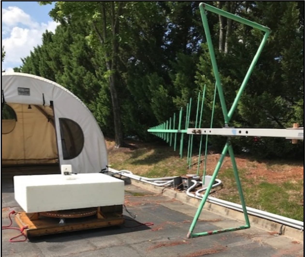
Photograph 2: Radiated Emissions Testing – Front View (Below 1 GHz)
