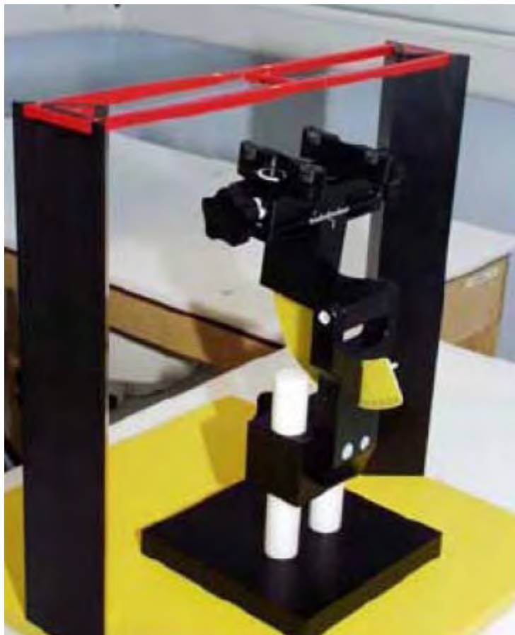
Figure 7 T-coil Phantom & Device Holder
