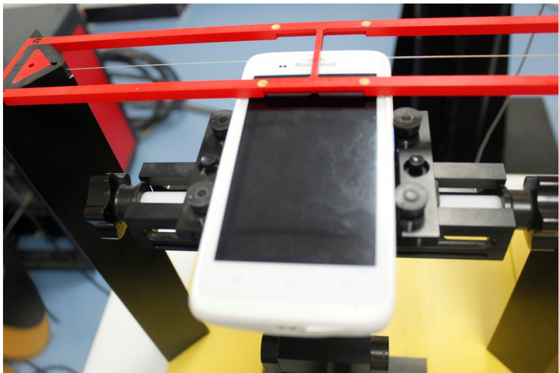
Picture 2: EUT Positioning for RF/T-coil
