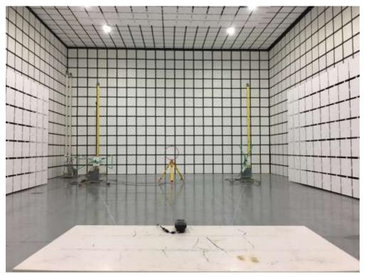
Description: Radiated Emission Test Setup for 30MHz~1000MHz
