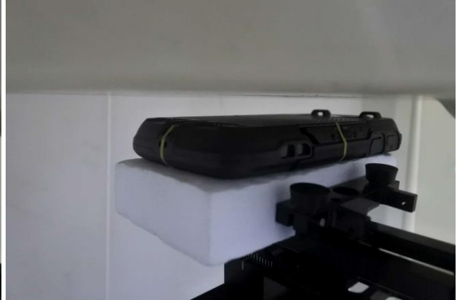
Rear Face, Test Separation 10 mm
