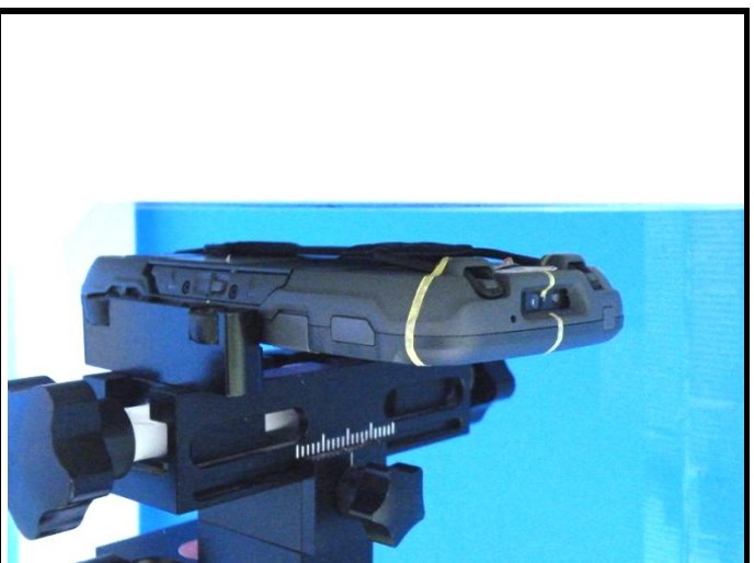
Body worn - Rear Face of EUT at 10 mm
