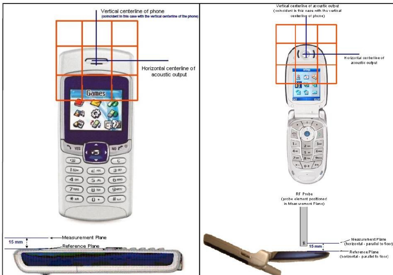
Fig-3.4 EUT Reference and Plane
