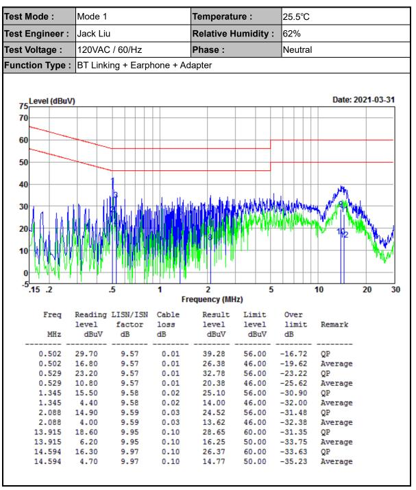
Result Level= Reading Level + LISN Factor + Cable Loss
