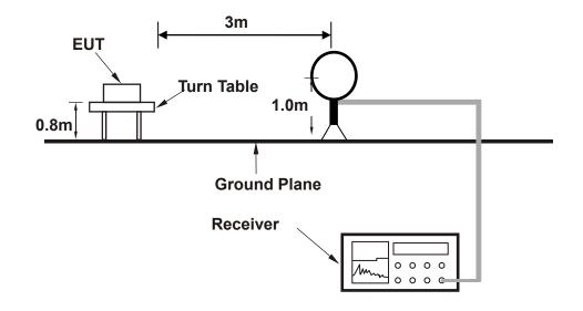
Setup diagram for Raidation(Below 1G) Test
