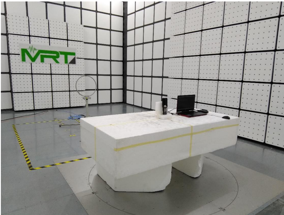
Description: Radiated Emission Test Setup for 9kHz~30MHz
