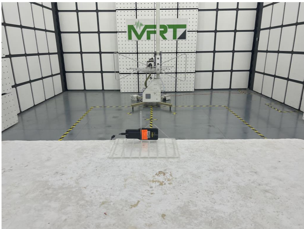
Description: Radiated Spurious Emission Test Setup for 30M ~ 1GHz
