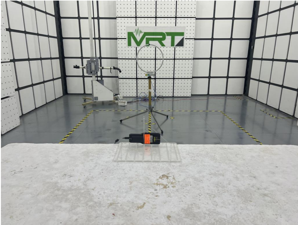
Description: Radiated Spurious Emission Test Setup for 30M ~ 1GHz
