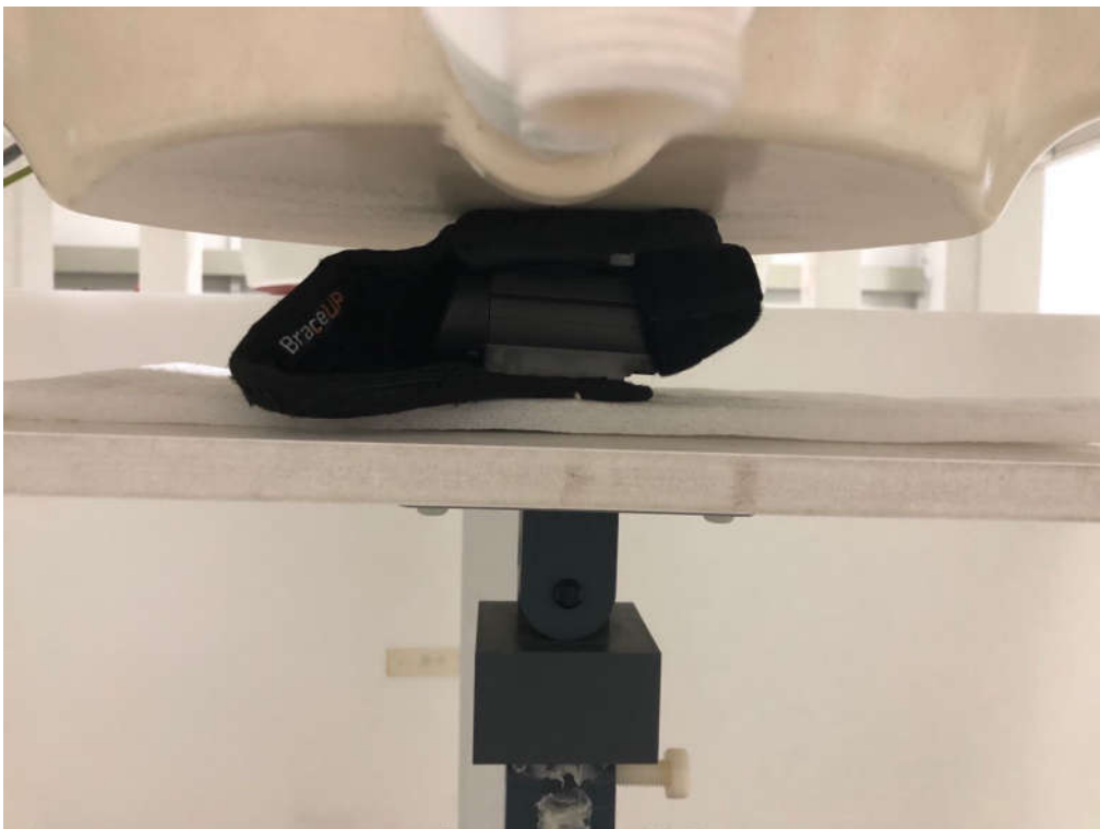
Description: SAR Test (Bottom)
