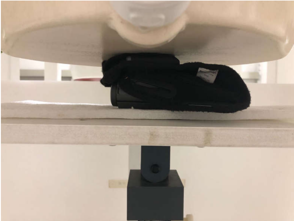
Description: SAR Test (Front)
