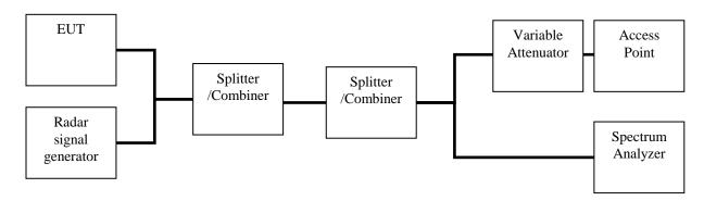
For The measurements at 20MHz and 40MHz channel bandwidth the DUT was connected via 50Ohm conducted port to a CISCO AP (AIR-AP1262N-A-K9) with FCC ID: LDK102073. Traffic was stimulated via pinging the EUT through an Ethernet connection at the access point.
