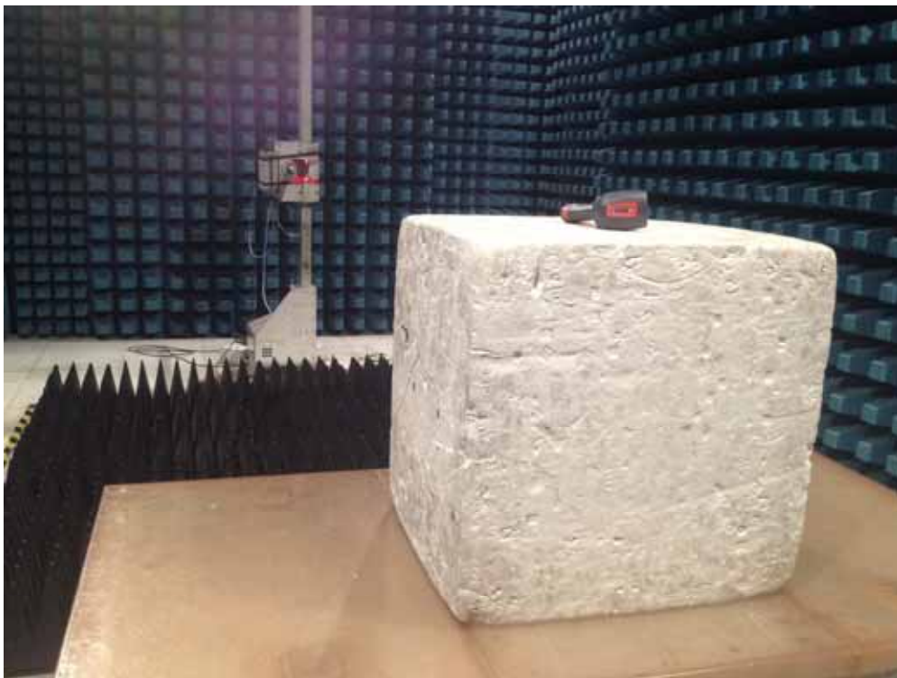
Description: Radiated Emission Test Setup for 1~18GHz
