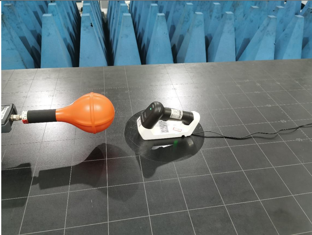
Description: RF Exposure Setup (Above 100kHz) - FCC
