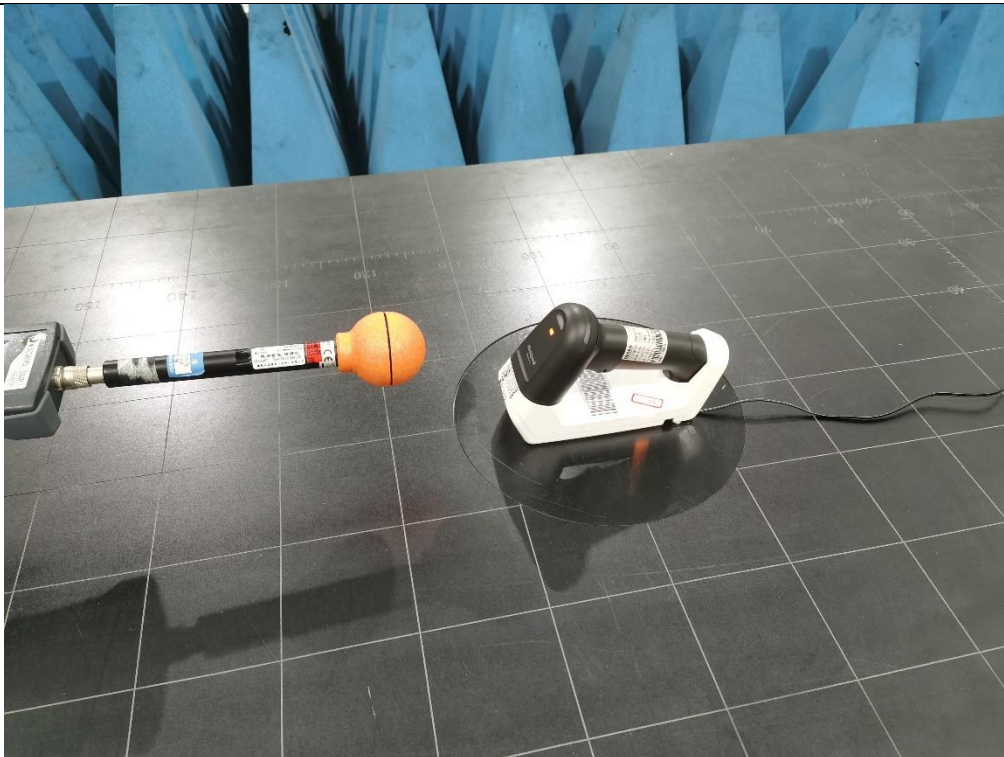
Description: RF Exposure Setup (Above 100kHz) - FCC
