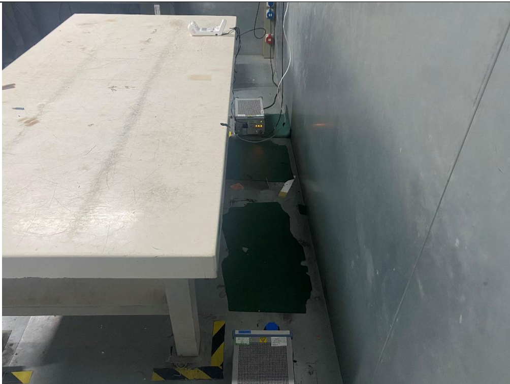
Description: AC Power Line Conducted Emission
