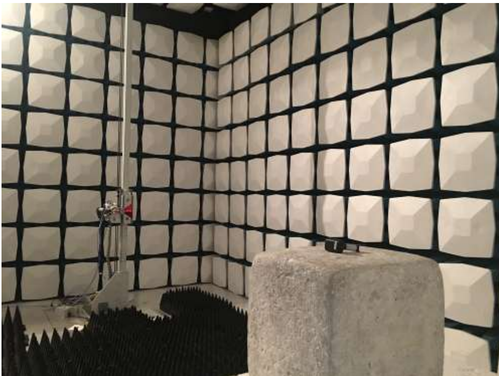
Description: Radiated Emission Test Setup for 1~18GHz
