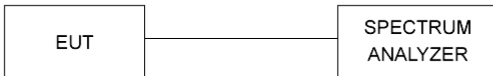
Figure 1 - Bandwidth Measurements Test Setup
