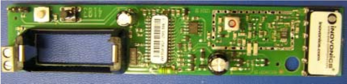
Photograph of the FA-250M board with the shield removed.
