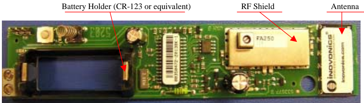
Photograph of an FA-250M board with the shield in place. Note PC mounted antenna is at the far right end of the board.
