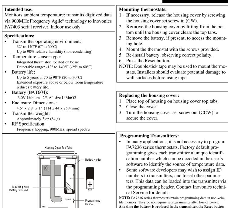
Any time the battery is replaced in the transmitter, the Reset button should be pressed to re-initialize the transmitter and to restore the most recent programming.
