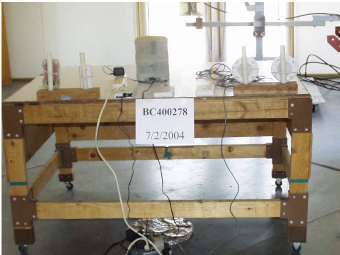
Test-setup photo(s): Radiated Unintentional Emissions
