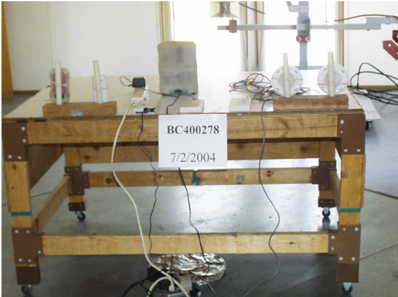
Test-setup photo(s): Radiated Unintentional Emissions
