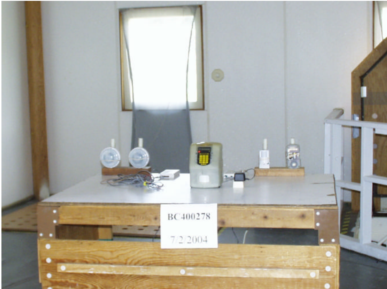
Test-setup photo(s): Radiated Unintentional Emissions
