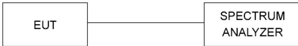
Figure 1 - Bandwidth Measurements Test Setup
