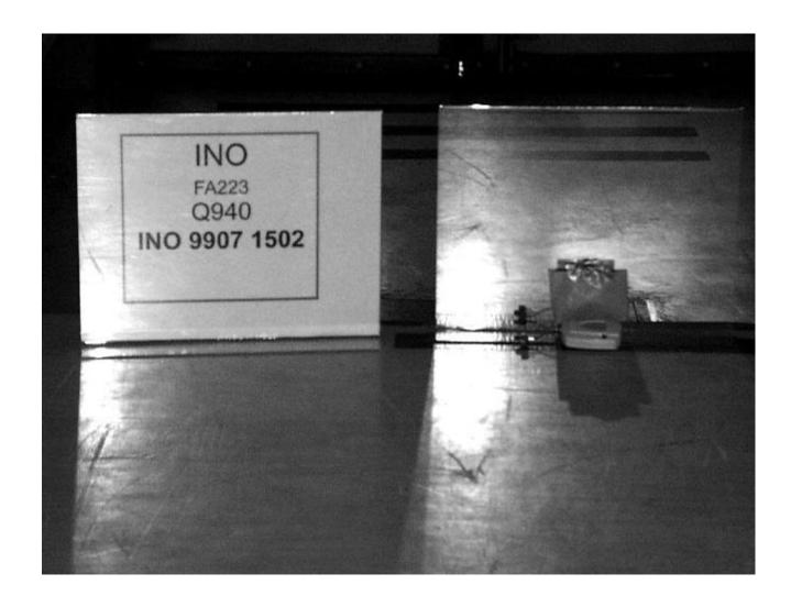
**Part 3.2 Radiated Emissions Orientation 2 Setup - Front View**
