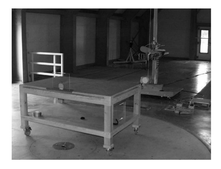
Part 3.5 Radiated Emissions Setup, 30 to 1000 MHz - Rear View
