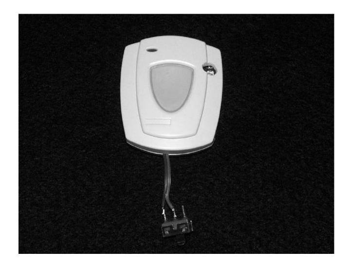
**Note:** The toggle switch is not a part of the production version of this device. It was used to enable the three frequency continuous hop sequence used during the test (fo low, mid, and high).
