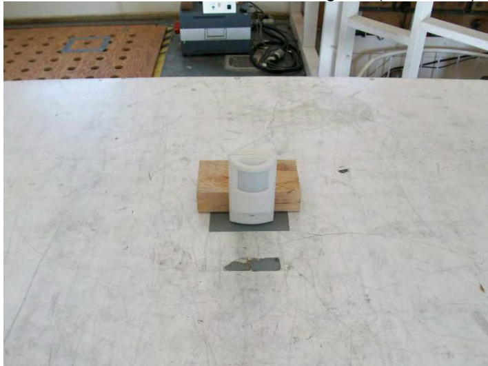
Axis 3 - EUT Vertical & Rotated 90 degrees (worst-case)
