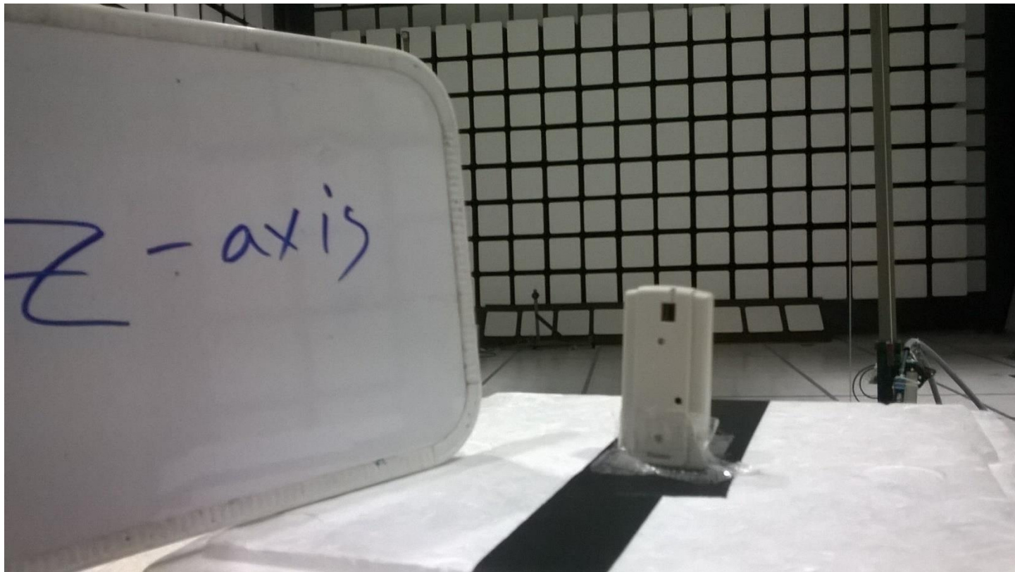
Figure 3 - Radiated Emissions Test Setup, 1 - 25 GHz, z-axis
