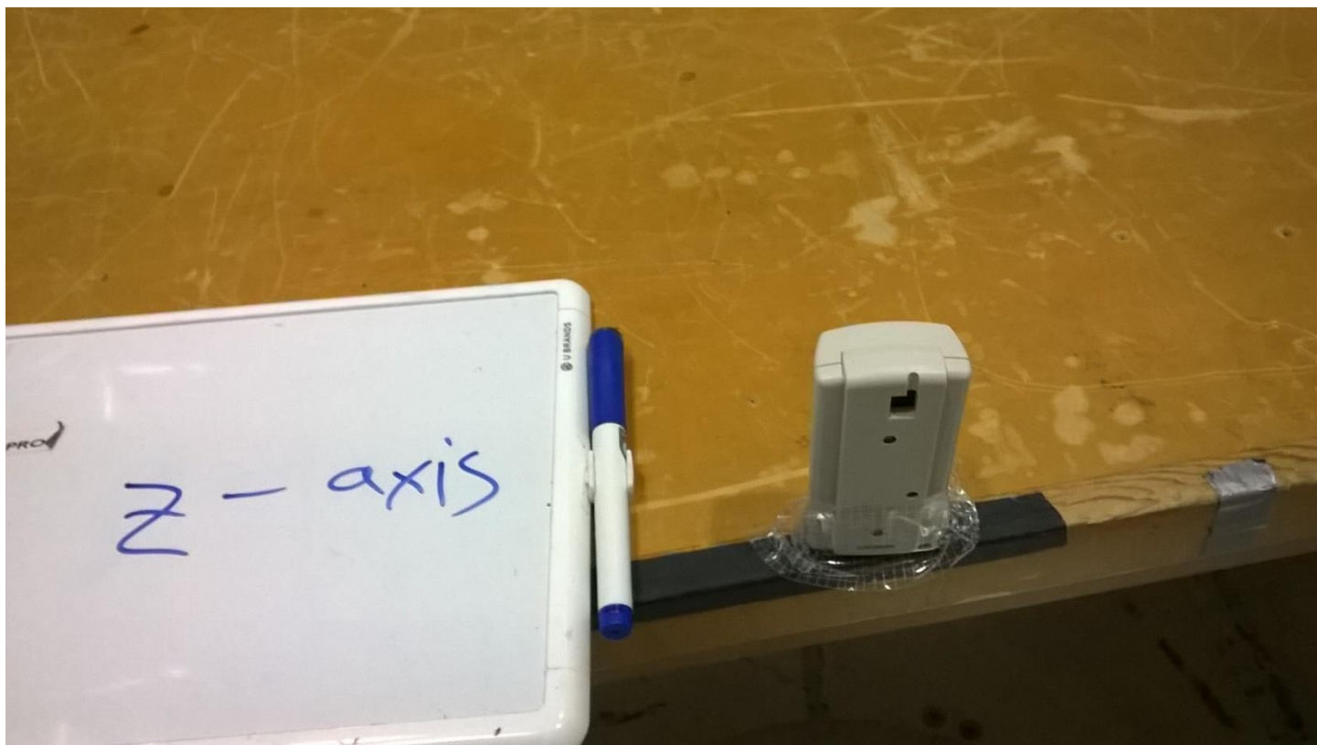
Figure 7 - Test Setup Photos, 30MHz - 1GHz, Z-axis
