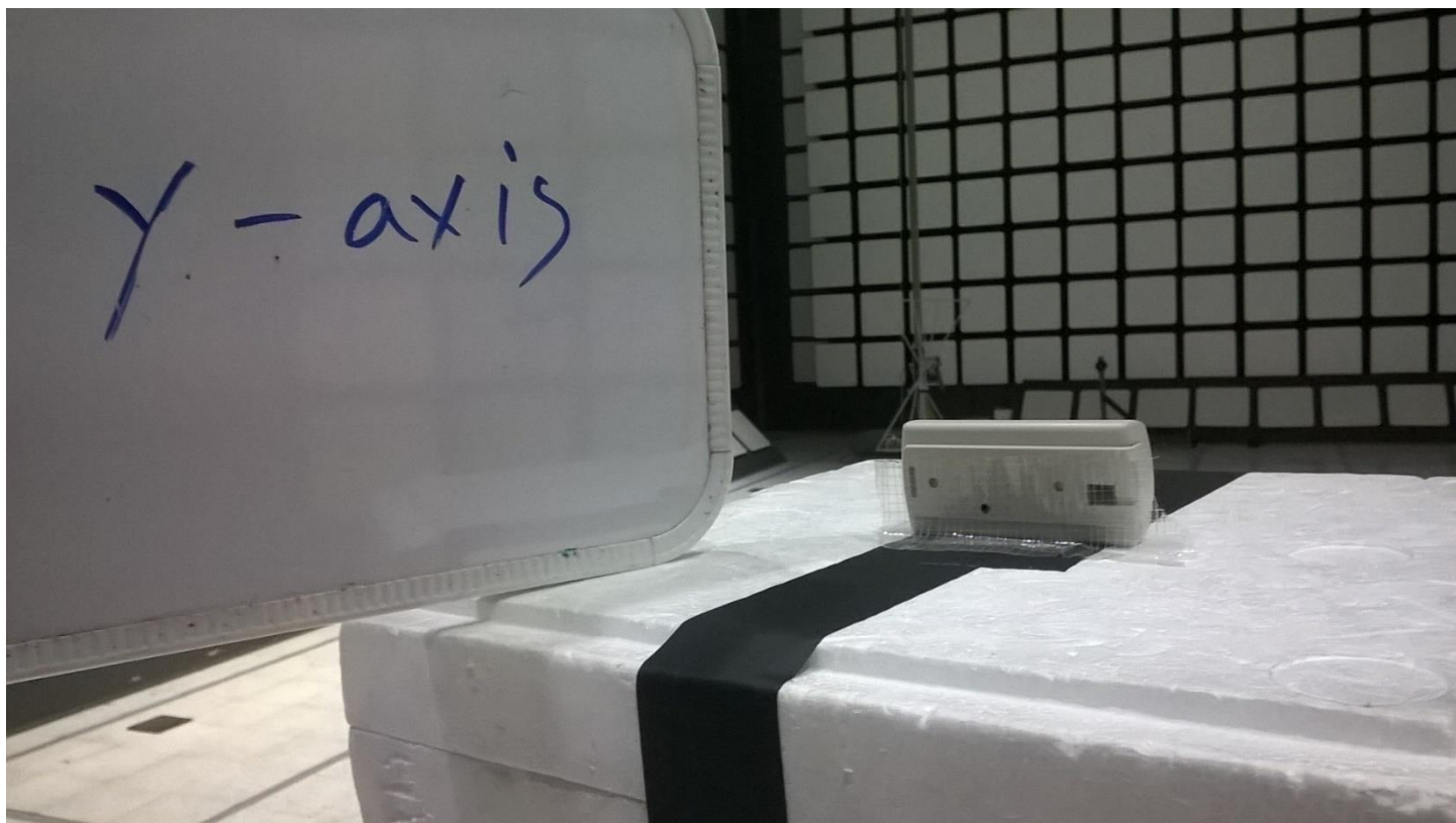
Figure 2 - Radiated Emissions Test Setup, 1 - 25 GHz, y-axis
