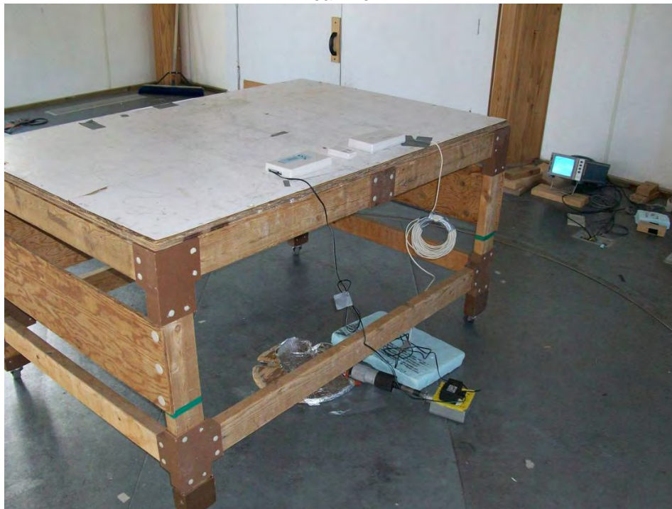
Pendant Transmitter located in center of table
