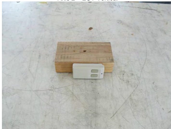
Axis 3 – EUT Vertical & Rotated 90 degrees (worst-case)
