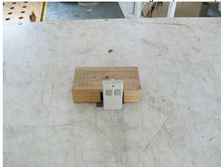
Axis 3 – EUT Vertical & Rotated 90 degrees (worst-case)
