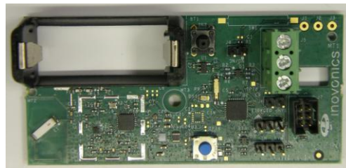
Picture 2 - EN1252 Top View Shield Can Removed
