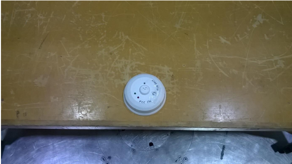
Figure 5 - Radiated Emissions Test Setup, Z-axis
