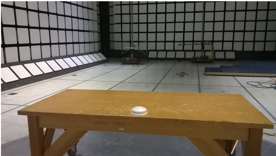
Figure 2 - Radiated Emissions Test Setup, 30Mhz – 1GHz
