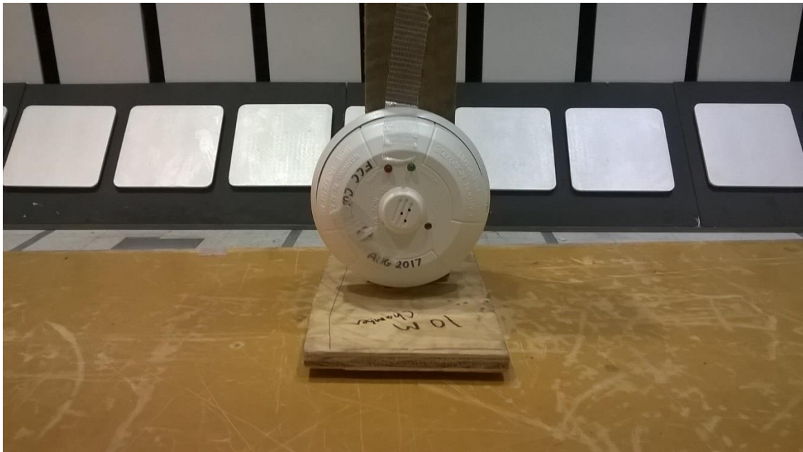
Figure 4 - Radiated Emissions Test Setup, Y-axis
