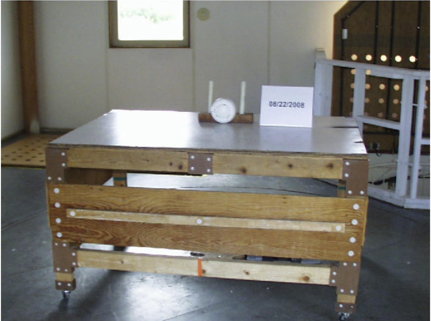
Test-setup photo(s): Radiated Intentional Emissions: Worst-Case Axis 3
