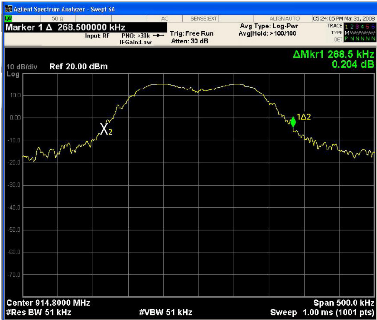
Plot 3: Demonstration of occupied bandwidth.
