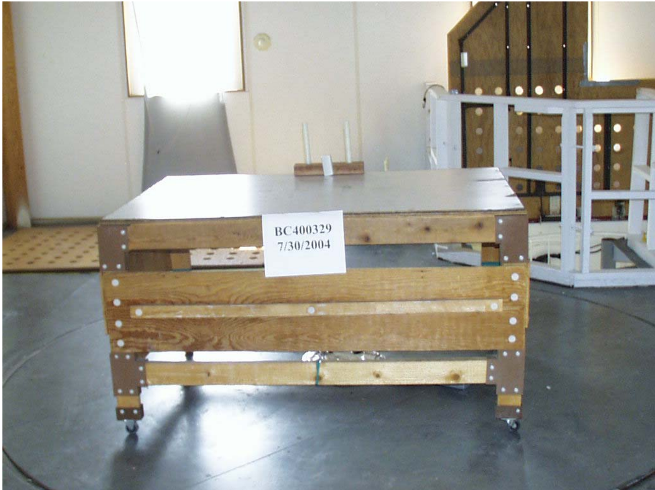
Test-setup photo(s): Radiated Unintentional Emissions
