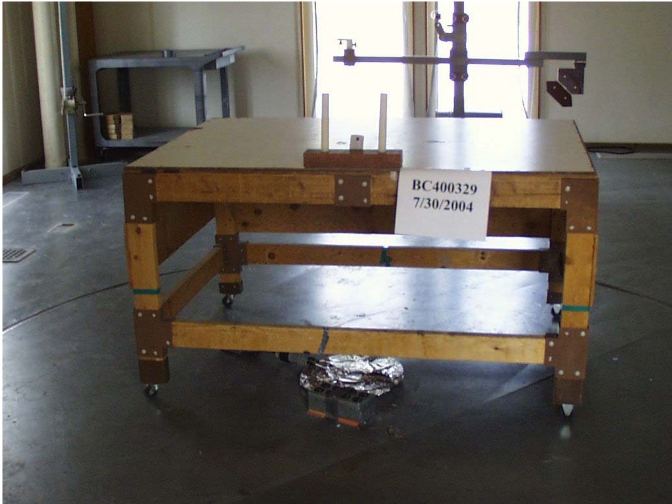
Test-setup photo(s): Radiated Unintentional Emissions
