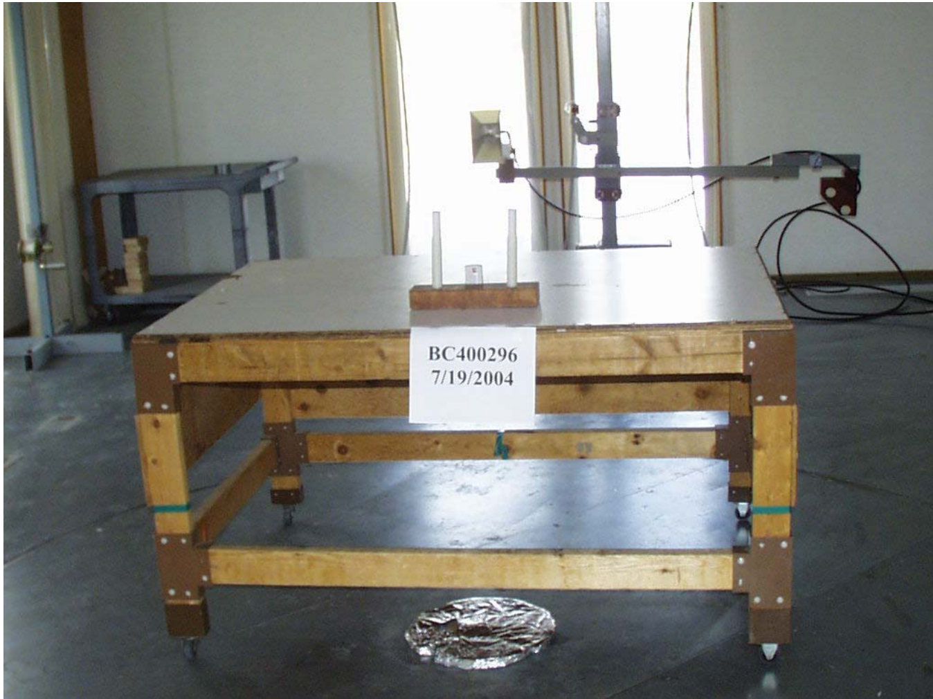
Test-setup photo(s): Radiated Intentional Emissions
