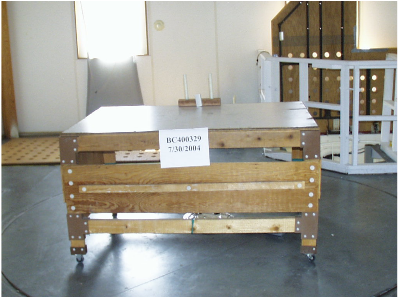
Test-setup photo(s): Radiated Unintentional Emissions
