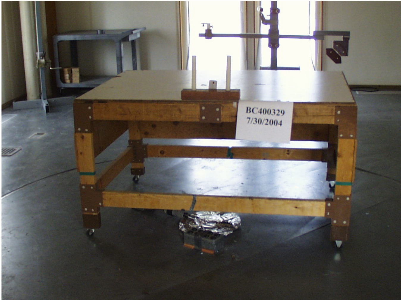
Test-setup photo(s): Radiated Unintentional Emissions
