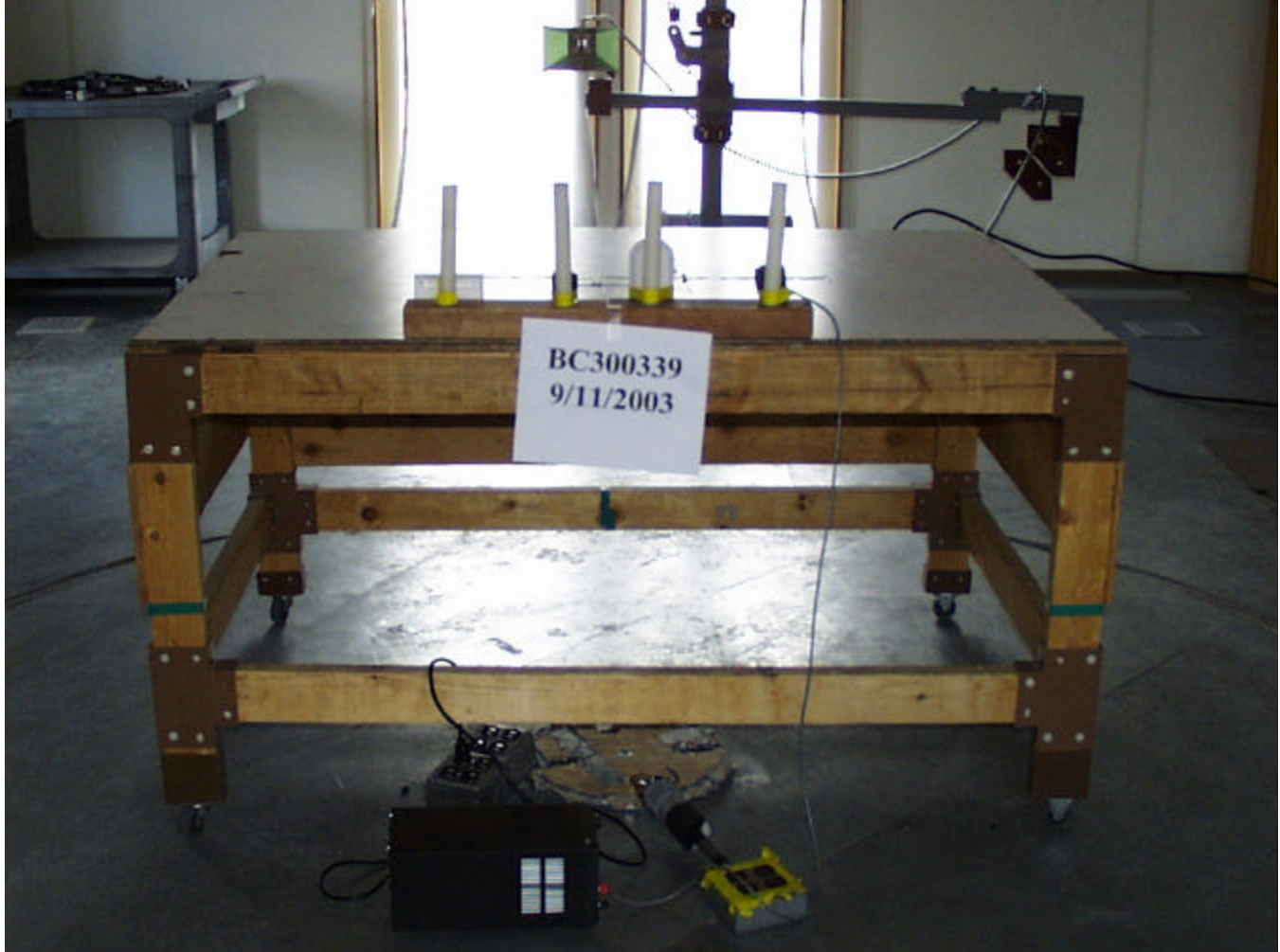
Test-setup photo(s): Unintentional Radiated Emissions
