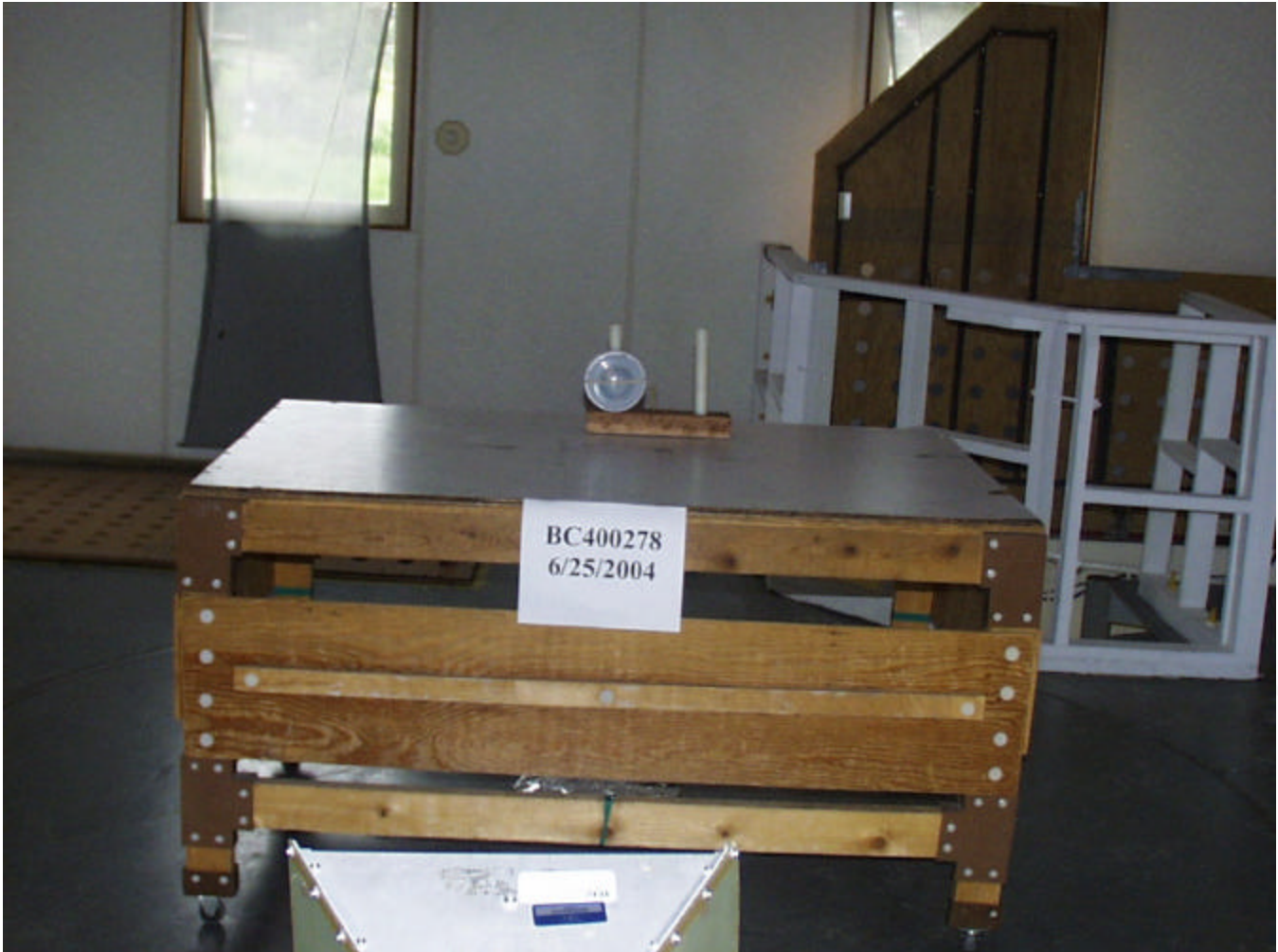
Test-setup photo(s): Radiated Intentional Emissions
