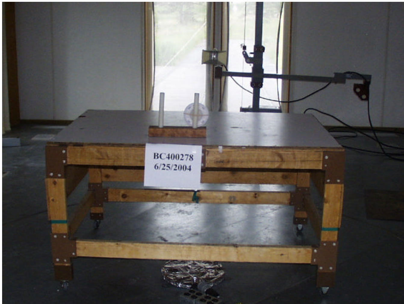
Test-setup photo(s): Radiated Intentional Emissions
